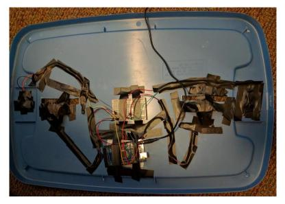
After I got the back-and-forth motion working, I still had to figure out how to get the heads to go up and down. After spending many hours trying to get the solenoids to work, my friend suggested that I use string to create tension on the head when the base moves. I tried their suggestion and, sure enough, it worked.
