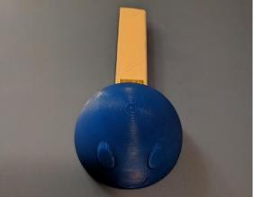
After that I started working on how I was going to make the head move up and down. I originally planned on doing this by connecting a copper pipe to the back of the hippo head and using a solenoid to pull on this pipe which would in turn pull on the head. However, the solenoid did not have enough force to do this.
