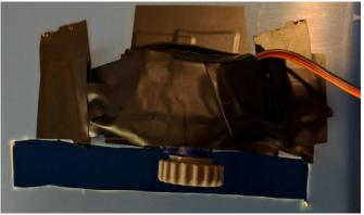
After getting the servos in place, I had to wire everything. I decided that the servos would be triggered using pushbuttons. I used an Arduino Mega to program my circuit and a lot of electrical tape to hold everything in place. I used a 9V power supply to power my circuit.
